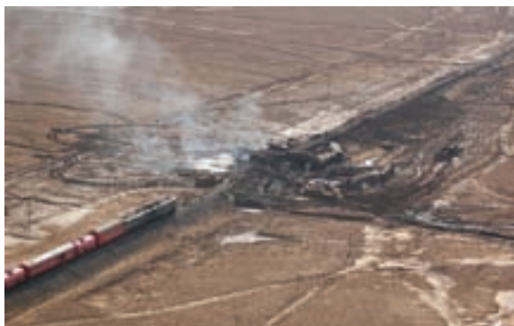
A Russian Fire Train at a rail incident. It is very much a one-shot response in terms of water and foam, similar to an airport crash rescue tender. Once the agents are expelled, refilling is back at the station.
