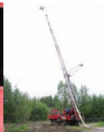
This aerial ladder lost its hydraulic power during an exercise requested by the author. Note the "engineers" working on the hydraulics. The "engineer" used a broom handle in an attempt to correct the defect, but the ladder was still in the same elevated position 24 hours later.
