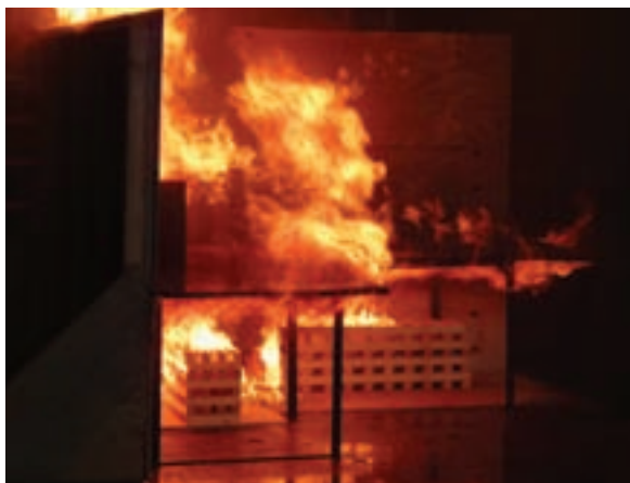
Inside BRE's test hall, where a watermist experiment was demonstrated using an office scenario developed in-house.
