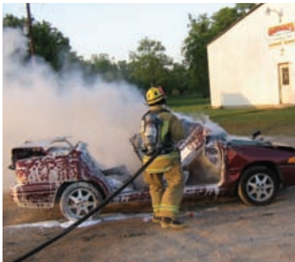
A change in the smoke from black to white is a good indicator that the CAFS is working.
