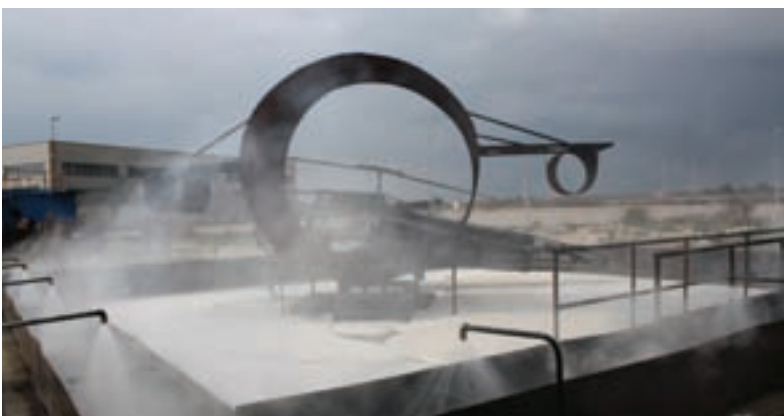
Full-scale test using a fire on a floating roof tank and Tema Sistemi's new low pressure watermist system Aquatech Plus, which uses a mixture of water and F-500.
