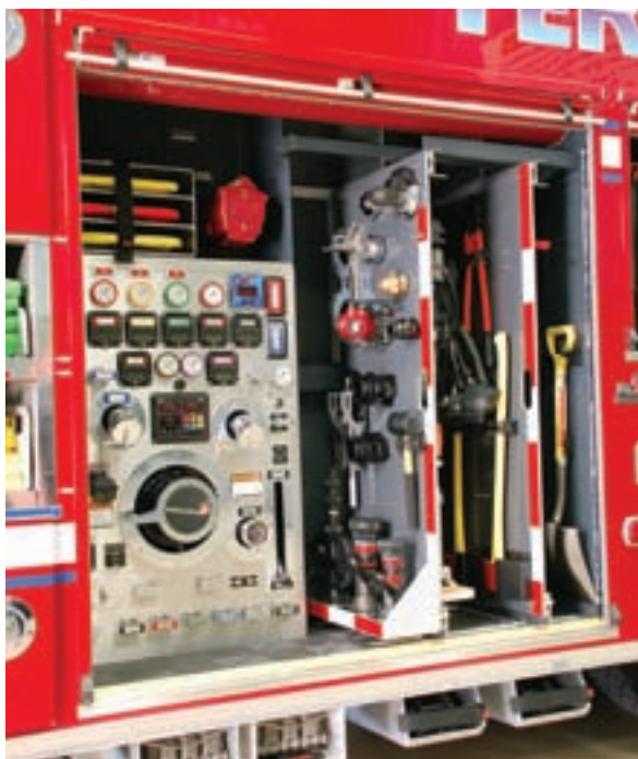
The Hale QMAX 2,000GPM pump features two 1.75-inch and one 2.5 inch speedlays for hose deployment.
