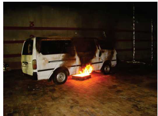
Figure 5. A pool fire located under the vehicle
