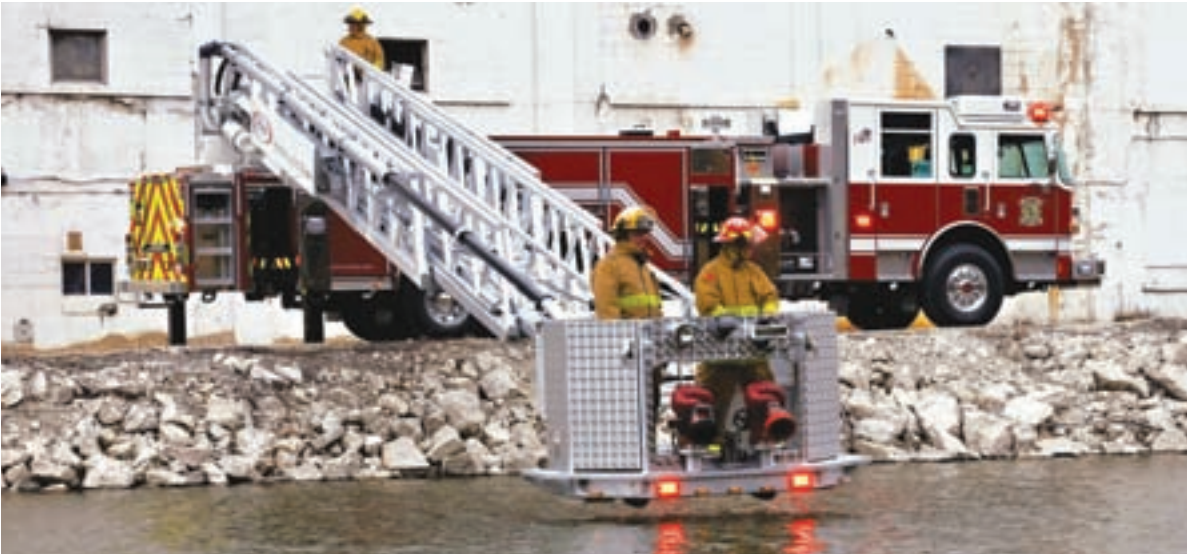
The Pierce 100-foot aluminum aerial platform features a small overall footprint that includes an 11-foot nine-inch overall height and a compact 15-foot six-inch stabiliser spread with 18 inches of ground penetration.
